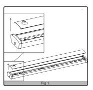
Remove the diffuser lens by using the supplied suction cup to lift up one end of the lens from the supporting channels.
