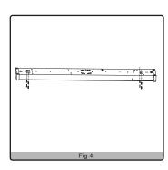
5. Re-install the reflector then apply diffuser lens by seating both sides of one end into each of the extruded channels and carefully press each side as you make your way down the length of the housing until it is fully seated.
