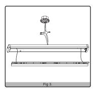
4. If wires are connected behind the fixture, carefully tuck the wires and wirenuts into the junction box before mounting the fixture. Align the fixture with the four (4) mounting screw heads so that the screw heads pass through the center part of the keyhole slots, slide the fixture to either side so that the screw heads are supporting the narrow slots of the keyhole profile.
