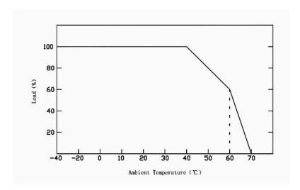
Make sure to adjust the load based on the load derating curve, which accounts for changes in ambient temperature. This helps prolong the working life of the system.
